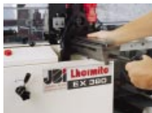
Tooling changes are quick and easy. Heavy duty tempered steel dies feature guide posts for perfect alignment, quick pin access and flanged holes to help waste clear out and add longer life.
