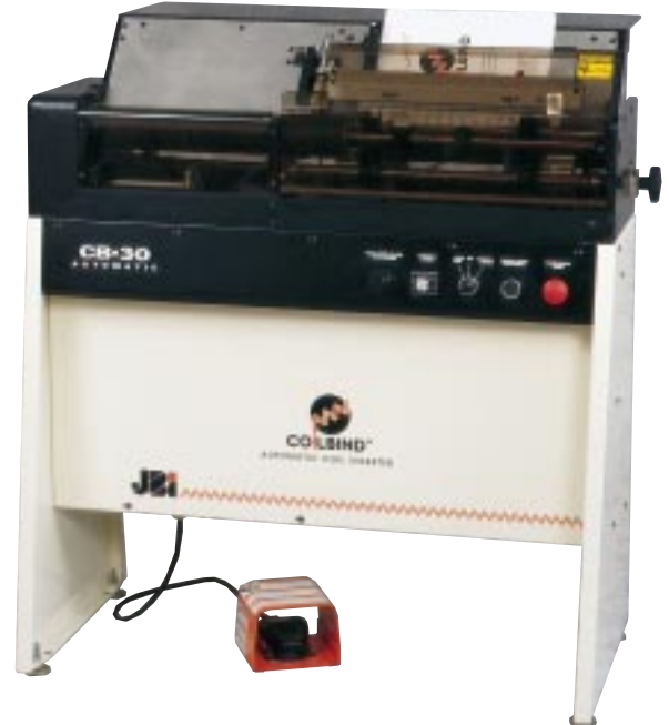
Position coil & depress foot pedal to quickly wind coil into book
