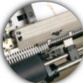
Position coil & depress foot pedal to quickly wind coil into book
