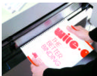
Most operations automatic - operator simply places prepunched sheets on wire elements.
