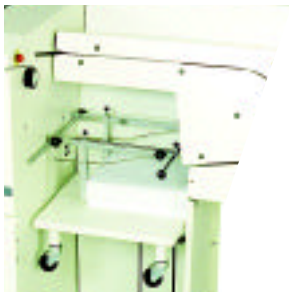
Unique turnover device keeps pre-collated work in perfect order, with Receding Stacker.
